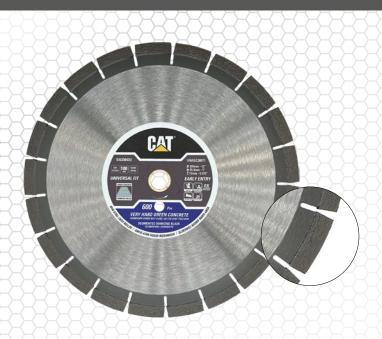
Cat® 600 Pro Very Hard Green Concrete laser welded diamond blades have a unique designed matrix with superior grade diamond grit designed to cut hard aggregate green concrete. The arbor is designed with a "snap out" section allowing the operator to choose from the triangular arbor or 25.4mm (1") size for use on multiple machines. Very neat cut, long life & good cutting speed.
