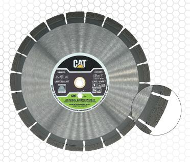
Cat® 600 Pro Universal Green Concrete laser welded diamond blades have a unique designed matrix with superior grade diamond grit designed to cut all types of green concrete. The arbor is designed with a "snap out" section allowing the operator to choose from the triangular arbor or 25.4mm (1") size for use on multiple machines. Very neat cut, long life & good cutting speed.
